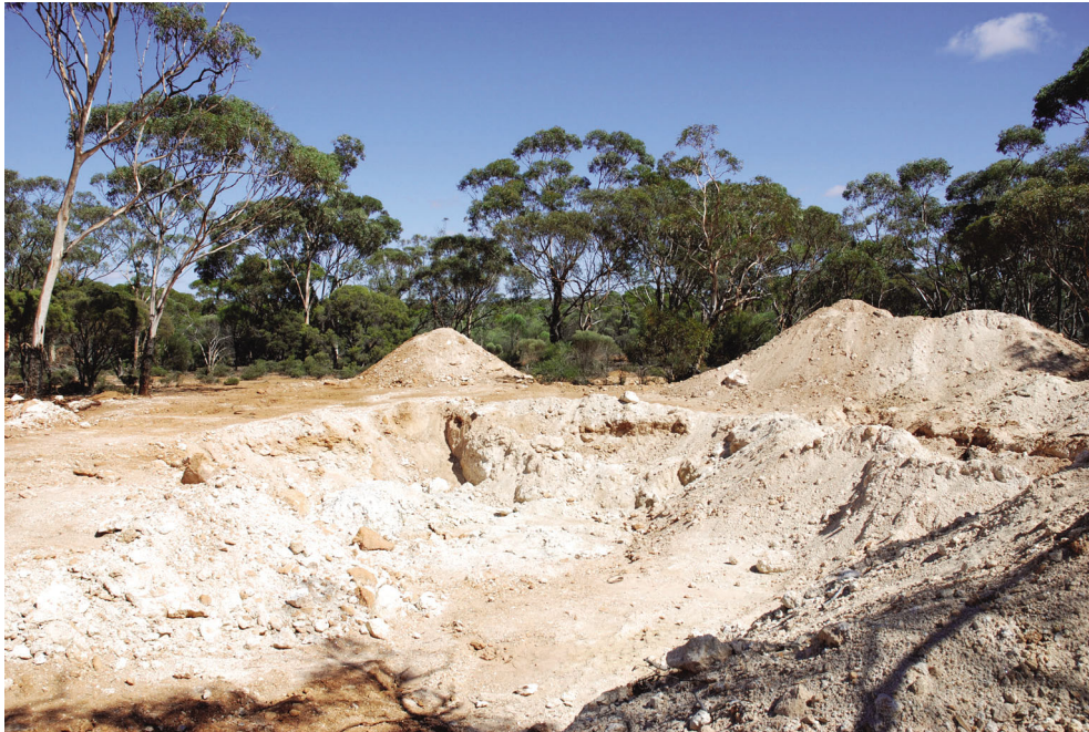
Figure 7.3 The Dalglish prospect in the Spargoville area has produced green and blue gem-quality elbaite tourmaline. The exploration pit is approximately 12 m in diameter x 1.6 m deep (courtesy Francine Payette)
